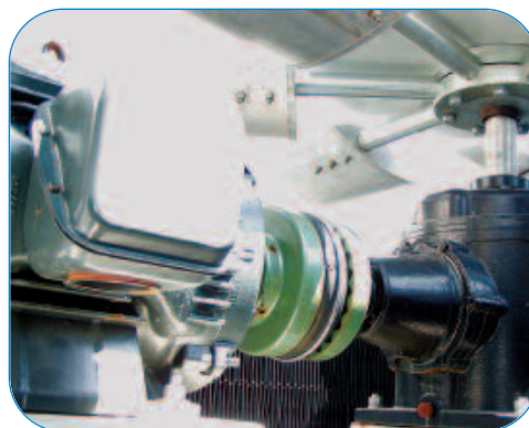
Gear drive system, close-coupled motor
