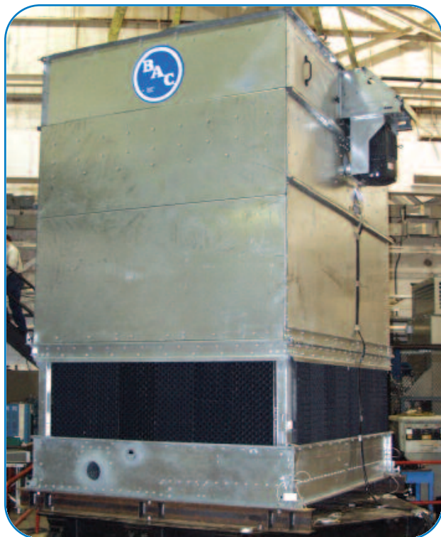
PT2 Cooling Tower Seismic Testing
